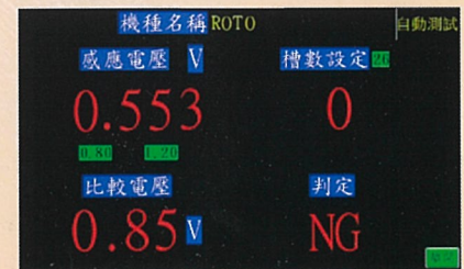
鋁棒斜角不良 (SKEW difference detection) 鋁材質不良 (Poor quality of aluminum alloy)
