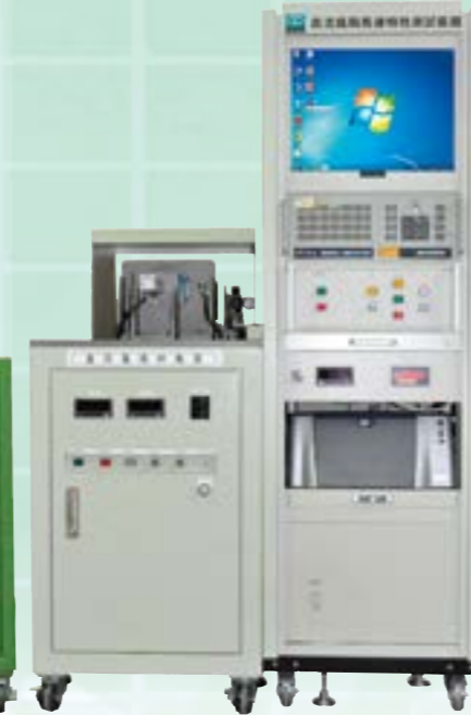
直流風扇馬達特性測試設備 Cooling Fan Motor Performance Test Equipment
