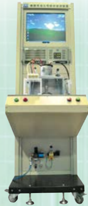
無刷馬達反電動勢量測裝置 DCBL Motor Back EMF Test Equipment
