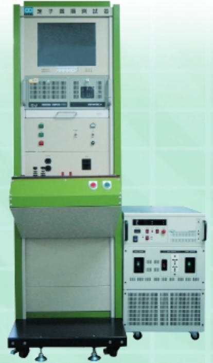
鐵損測試設備 Stator Loss Test Equipment
