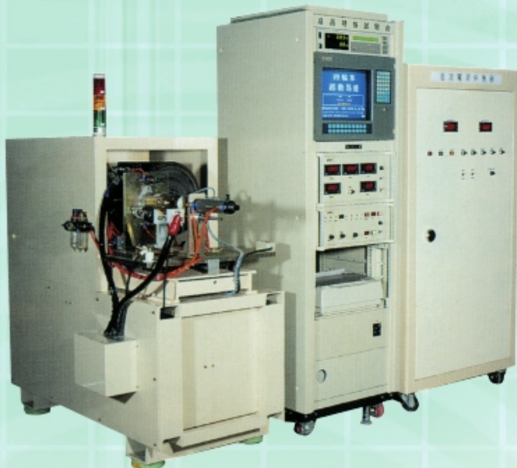
汽車起動馬達特性測試設備 Car Starting Motor Characteristic Test Equipment
