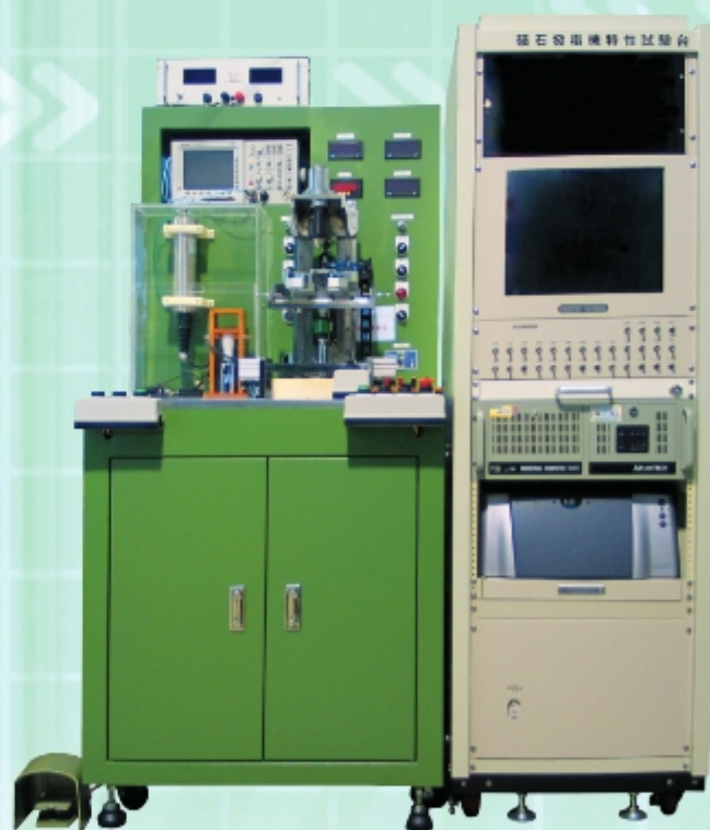
ACG 磁石發電機測試設備 Motorcycle AC Generator Characteristic Test Equipment
